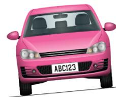
The angle of the plate should not exceed 5° (clock or anti clockwise).
